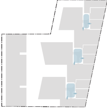
9. The naturally ventilated lightwells provide opportunities for secondary natural ventilation and light.
